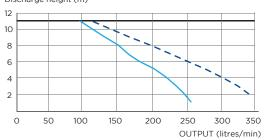
P1 - Output flow rate with one motor engaged P1 + P2 - Output flow rate with two motors engaged
