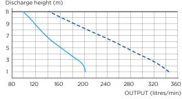
P1 - Output flow rate with one motor engaged P1 + P2- Output flow rate with two motors engaged
