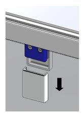
**16)** Slide the outside Clamp Block Covers off the Pivot Clamp. Using a flat blade screwdriver sufficiently loosen the two screws, adjust the door by sliding left or right in the pivot
