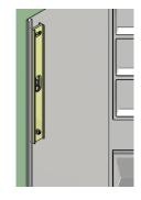
2) Plumb up the Door Wall Receiver using a spirit level. Mark the position with a pencil line.
