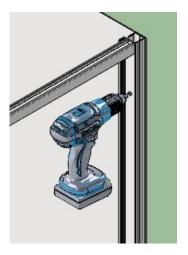
8) Plumb the Door and remaining Wall Receiver. Through the oversize holes in the Door jamb drill through the Wall Receiver frame and into the wall stud using a 3.0 mm drill bit
