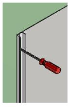
**4)** Secure the Wall Receiver to the wall using the No.6 x 38mm stainless steel screws
