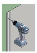
3) Pre drill three equally spaced clearance holes (i.e. top, bottom and centre) in the Door Wall Receiver using a 4.5mm drill bit. Reposition the Wall Receiver to the pencil line on the wall. Drill into the wall through the clearance holes using the 3.0mm drill bit. N.B. The holes preferably locate into a stud or nog. As an alternative, a toggle system can also be used.
