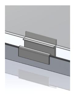
**7)** Ensure the Door is facing the correct way with the door opening outwards. Do not remove the door setting block, this will assist in supporting the door during installation and setting the correct clearance from the sill.
