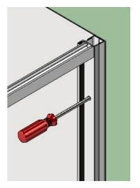
**9)** Secure the Wall Receiver to the wall using the No.6x 38mm stainless steel screws.
