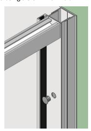
**10)** Cap the oversize holes in the door Jamb using the 9mm plastic plugs
