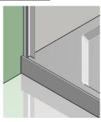
Determine which side the Door is to be hung. Position one of the Door Wall Receivers hard against the inside edge of the tray upstand.
