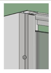
**14)** Secure in place using the 6 gauge x 10mm **15)** Cover all Screw heads with the Screw Caps screws.
