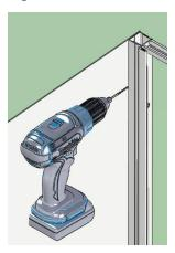
13) From the inside using a 3.0mm drill bit; drill through the vertical sections of the Door into the Wall Receivers. Fix the Door to the Wall Receivers. You must have a minimum of 10mm overlay and the holes must be drilled no less than 5mm from the edge of the vertical aluminium sections. Secure in place using the 6 gauge x 10mm screws.
