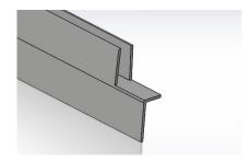
**17)** The Drip seal is supplied in a 1m length, this will need to be cut to the desired lengths for each side of the pivot . The opening side Drip seal will also need to be notched to fit under the door magnet profile. Make the Notch 13mm in length and finishing down to the horizontal ledge of the drip seal
