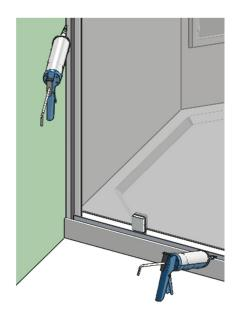
18) The Door can now be sealed in place using silicone sealant. Ensure all surfaces are first cleaned with dry clean cloth. Seal between the tray upstand and the door set along the bottom outside edges. Seal vertically between the Wall Receivers and Wall Liner
