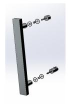
5) Fit the handle to the door (where required). This will assist in the opening & closing during the installation process
