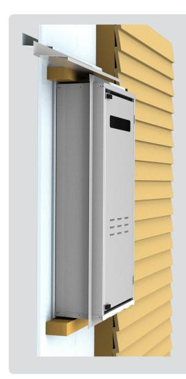
These instructions are a guide only, designed to be used in conjunction with the NZ Building Code Approved Document - External Moisture E2. The recess box installation can be compared to the detail required to install a meter box.
